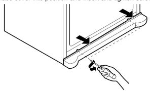
Turn the leveling screw clockwise to raise that side of the refrigerator or counterclockwise to lower it. It may take several turns of the leveling screw to adjust the tilt of the refrigerator.
